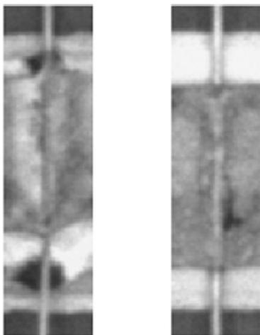
Figure 4: 10,000-pixel images of two soldered wires (b = Good, c = Bad). Question: has the solder flowed, or are the components only mechanically connected?
