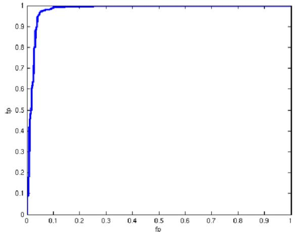
Figure 5: ROC curve of the SVM separation function.  $\Sigma = 2$ ,  $C = 1$  in this object space  $\rightarrow$  test error 4.01%
