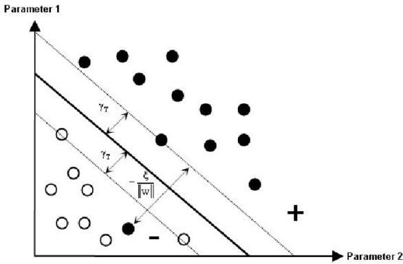
Figure 2: Linear separation of a two-dimensional data set with a misclassification
